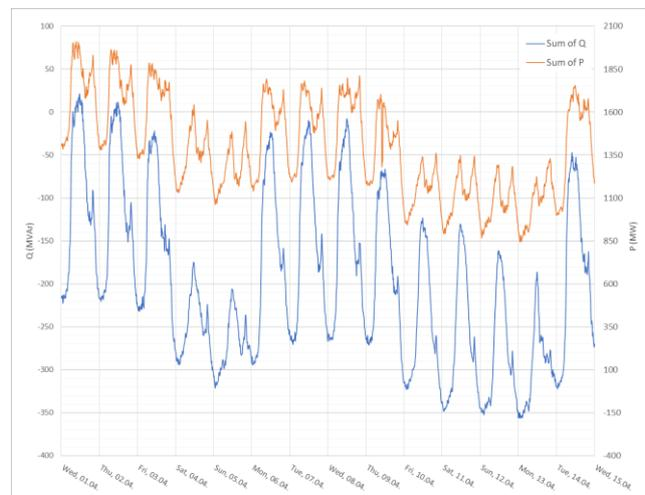
Figure 5 P and Q chart for the whole EG.D area over the Easter time, blue line represents  $Q$  and orange line represents  $P$
