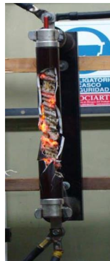
Fig. 25: Laboratory test of a low current operation failure of an aged HBC fuse
