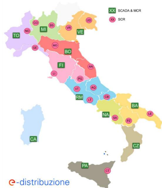
Fig. 14: Grid Area Subdivision, Server Farms, MCR and SCR (Paper 1341)
