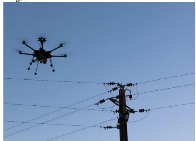
Fig. 5: UAV during an Aerial Power Line inspection
