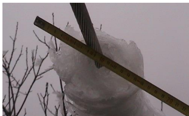
Figure 1 of paper 0279: Accumulated ice on an overhead line
