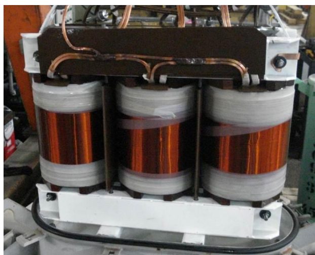
Figure 4 from paper 1078: Core and coil assembly immediately after untanking
