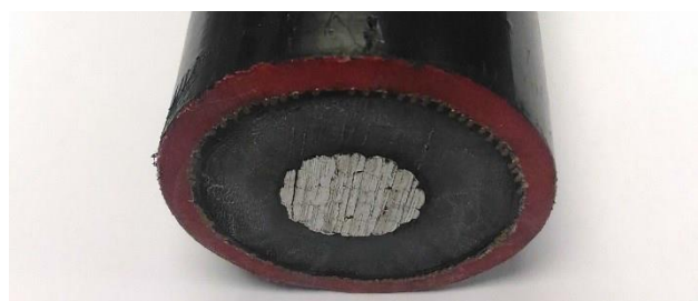
Figure 4 of paper 0266: MV insulated cable sample with external conductive layer and red colored over-sheath
